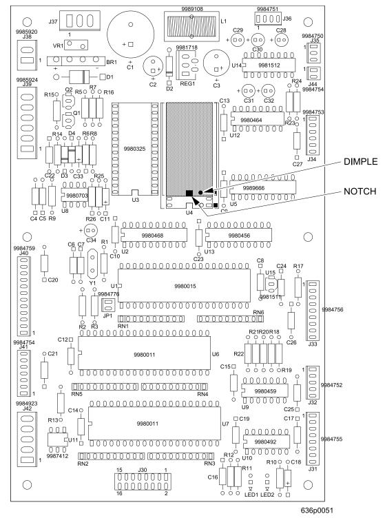
Figure 18 Controller Card Showing the Location of EPROM U4
